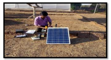
Fig. 1 Testing of SPV panel with fixed angle
